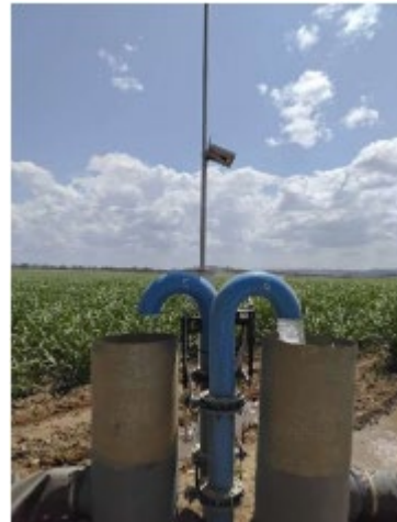
LEFT: Base station and computer for the WiSA radio network and Farm in ONE platform. RIGHT: Radio field module controlling 2 valves delivering water to 2 irrigation sets.
