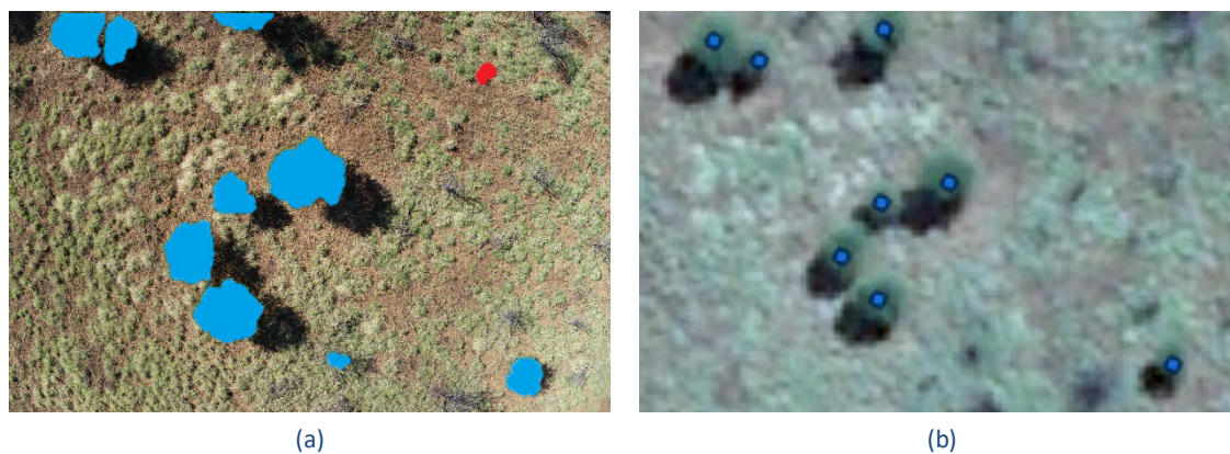
Figure 10: Using the sample image in Figure 6 to compare (a) drone-AI result with (b) satellite-AI result. The satellite-AI does not have a false positive detection on top-right (as drone-AI has). However, it has a false negative for not detecting the small Prickly Acacia in bottom-middle.
