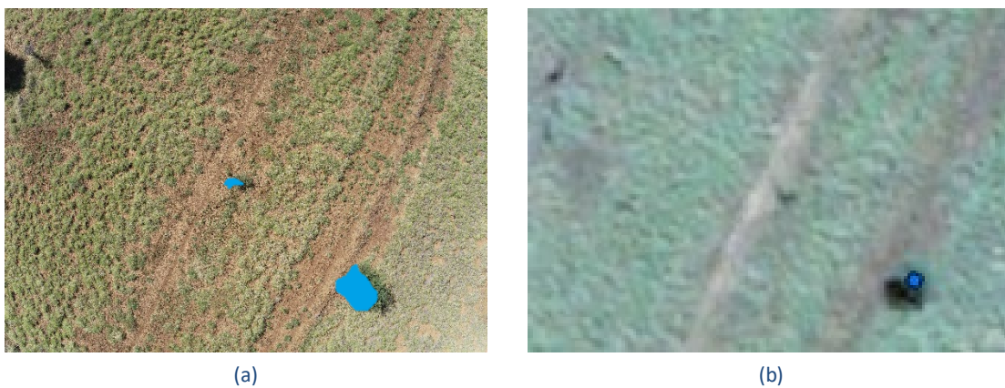
Figure 9: Using the sample image in Figure 4 to compare (a) drone-AI result with (b) satellite-AI result. Drone-AI has correctly detected the small tree in the middle of the image, but it was too small to be picked by satellite-AI.
